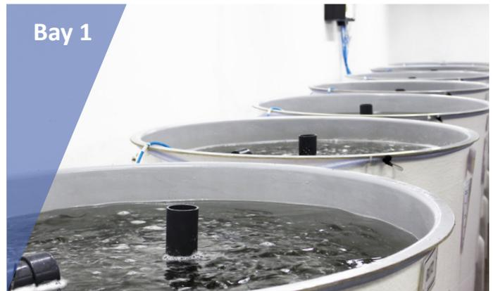
Eighteen (18) tanks in system (500 L each) with full RAS. The Bay can be operated for both feed or challenge trials. Freshwater or marine species system.
